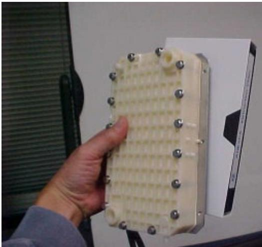
Electrolysis chamber from an Enagic water ionizer as compared to a standard VHS tape
