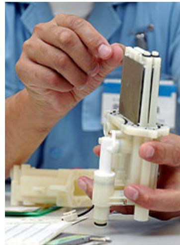
Electrolysis chamber plates from a Jupiter water ionizer not even the size of a playing card
